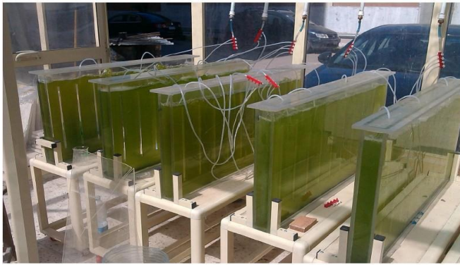
Algae Cultivated In Flat Panel Photo-Bioreactor, Med-Algae Project (Faculty of Science, Alexandria University)
