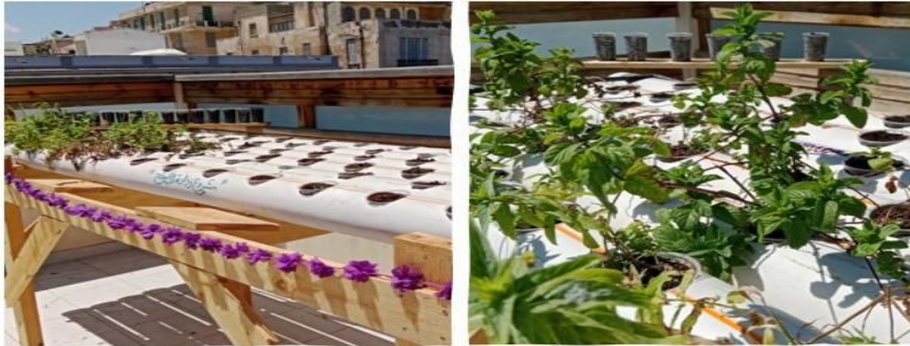
Grey water recycling system organized by Faculty of Pharmacy (Alexandria University, Egypt), and reused in rooftop cultivation.
