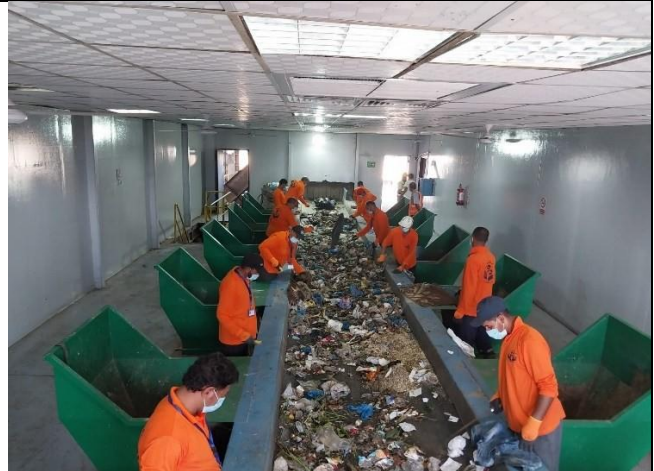
Manual sorting hall in Nahdet Misr company for waste collection in Alexandria
