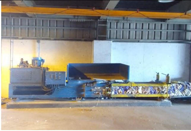
Paper and carton baler in Nahdet Misr company for wastes collection in Alexandria
